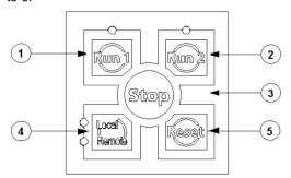
Control keys 1 to 3 are used to control LTM R outputs O.1 and O.2. The function of control keys 1 to 3 depends on the motor operating mode. The following table lists their functions for each operating mode:
